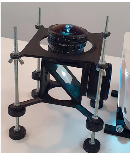
Figure 5: The projector system that is used inside the cardboard DIY planetarium.
