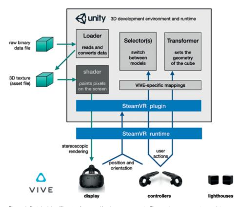
**Figure 4.** Sketch of the different software and hardware components. The grey boxes represent our scripts (written in C#, except the shader, which is written in Cg). The green arrows show the data flow when the full data cube is loaded for volume rendering. The blue boxes and arrows represent the SteamVR layer that interfaces Unity with VIVE; it takes care of stereoscopy and tracking and listens to user inputs. Credit: RIKEN/ABBL
