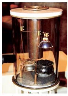
**Figure 4.** Experimental setup. The glass container with the sample is in a vacuum chamber; the liquid nitrogen trap is the copper cylinder in the middle of the chamber which is open at its top; and the halogen lamp is above the sample.
