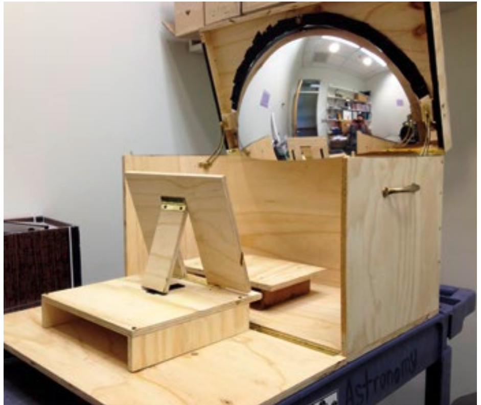
Figure 2. The optics box in the mobile planetarium. The do-it-yourself guide to building the above optics box is available on our website 4 .
