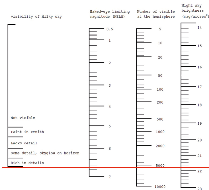
Figure 2: A nomogram comparing different night sky brightness measurements. The red horizontal line indicates the natural night sky unobscured by light pollution. Image Credit: After IAU (n.d.)
