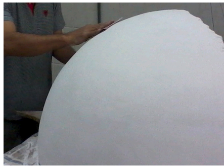
Figure 3. Spherical surface coated with plaster to remove imperfections. Credit: Aquino, H. A.
