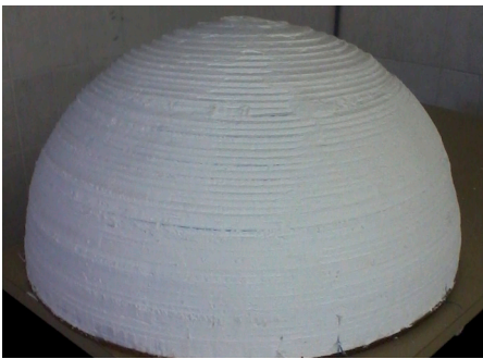
Figure 2. Photograph of a spherical surface made of Styrofoam stacking layers. Credit: Aquino, H. A.
