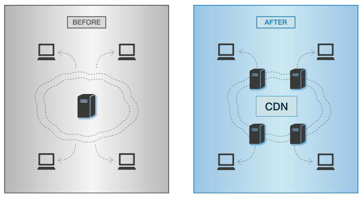
Figure 1. Comparison between content distribution from a single server (left) versus a content delivery network (right).
